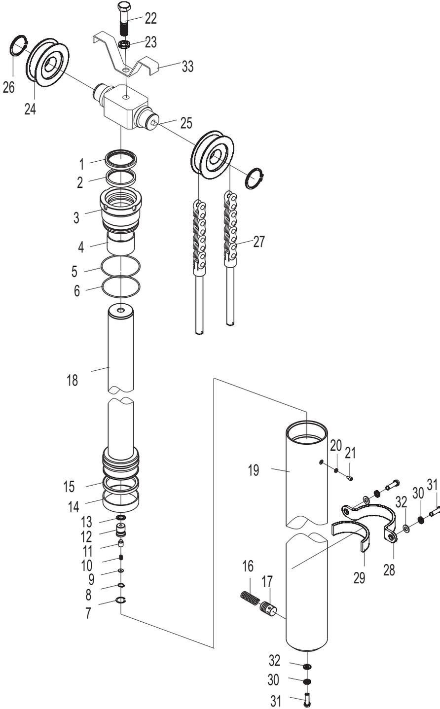
前起升油缸(三级全自由) / Front lift cylinder (full free 3-stage mast)
