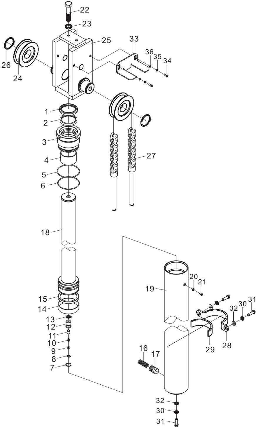
前起升油缸(二级全自由) / Front lift cylinder (full free 2-stage mast)
