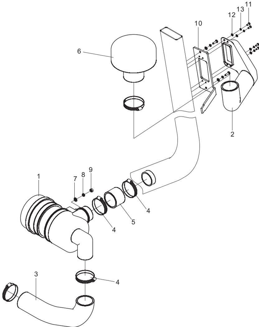
**空滤器总成(预滤器) / Air cleaner assembly(prefilter)**
